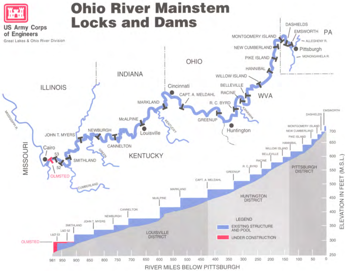
Figure 2 Location of the Ohio River Mainstem Locks and Dams (USACE), showing the Ohio River profile from Pittsburgh to Smithland Dam.
